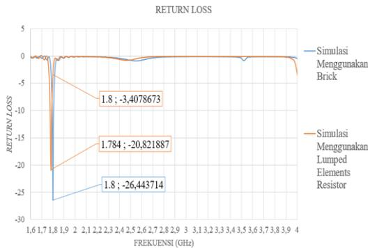
Gambar 9. Hasil Return Loss Kondisi On Brick Dan Lumped Elements Resistor.
