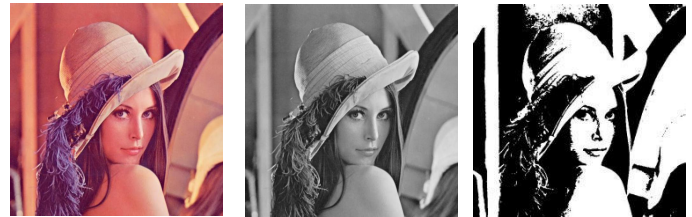
(a) (b) (c) Gambar 2.8 (a) citra warna (b) citra grayscale (c) citra biner
